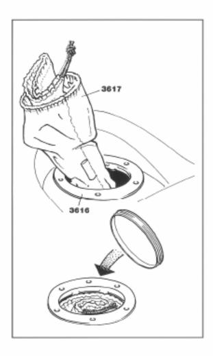
5 Insert the hatch bags [3617] inside the hatches adjacent to the mast.
