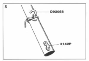
9 Tie the clew outhaul line to the small fairlead [3142P] fitting on the end of the boom with a bowline loop, then run through the eye of the clew hook, back round the fairlead and up to the cleat [2123] on the boom.
