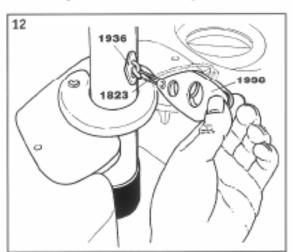
13 Take the small kicker block [1364] and fit it to the eyelet on the boom (near the front end), using the small pin and ring.
